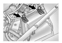
Lift the filter cover tabs on top of the engine air cleaner/filter housing.
